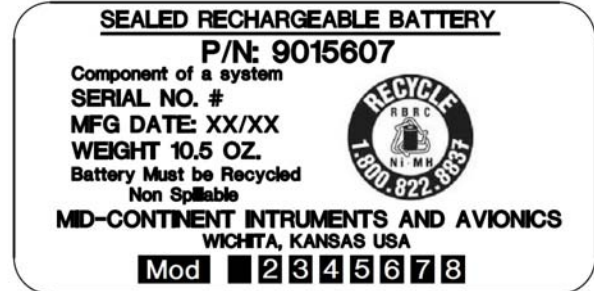
Figure 2.3 Standby battery Mod 1 nameplate
