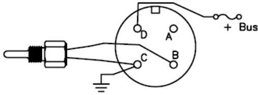
Mid-Continent MD11-6 gauge used in 28 volt system. Uses AN3106-14S-2S connector.
