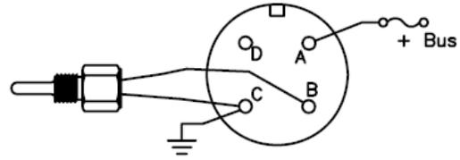
Mid-Continent MD11-3 gauge used in 12 volt system. Mid-Continent MD11-4 gauge used in 24 volt system. C-11, C-12, F-8, or F-9 gauge. 12 or 24 volts as indicated on dial. Uses AN3106-14S-7S connector.
