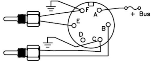
AN5790-6 or C10 gauge used in 12 volt system. Uses AN3106-14S-2S connector.
