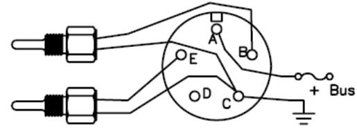
Sutton-Horsley Canadian gauge. Caution!! Not all S-H gauge types match AN specs. 12 or 24 volts as indicated on dial. Uses AN3106-14S-2S connector.
