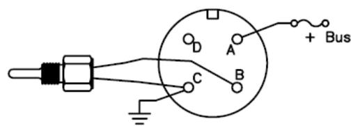
AN5795-6 Dual Gauge used in 12 volt system. Uses AN3106-14S-5S connector.
