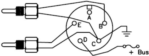
AN5795-6 Dual Gauge used in 24 volt system. Uses AN3106-14S-5S connector.
