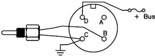
AN5790-6 or C10 gauge used in 24 volt system. Uses AN3106-14S-2S connector.
