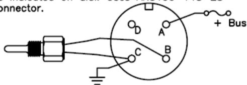
Sutton-Horsley Canadian gauge. Caution!! Not all S-H gauge types match AN specs. 12 or 24 volts as indicated on dial. Uses AN3106-14S-2S connector.
