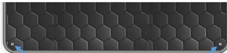
Punch holes with push pin to provide clearance for 2-56 screw
