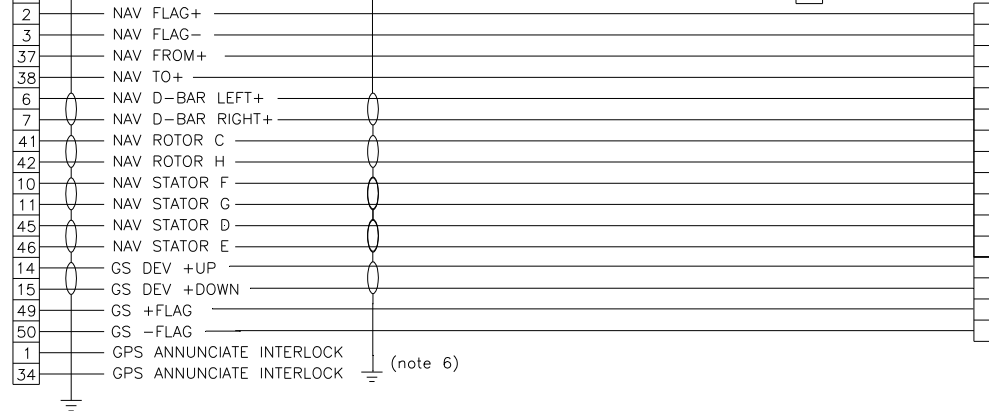
FIGURE 3-5 WIRING DIAGRAM, MD41-924A/934A KLN 900 (14V)
